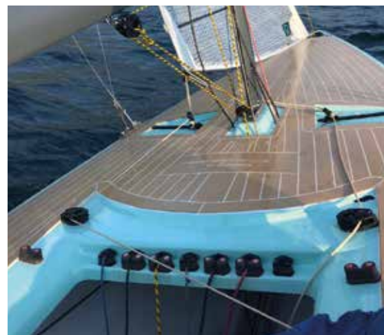
Plasdeck’s Performance 3.5 is a lightweight PVC decking designed for fast craft
