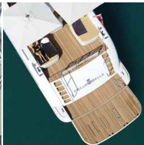
The different colours and textures available in PU extrusions allow for natural-looking decks. Here are two examples from UK-based Permateek, which reflect the two most common trends – a deck that has ‘matured nicely’ by ‘natural’ weathering (left) and a ‘just scrubbed’ teak deck (right)
