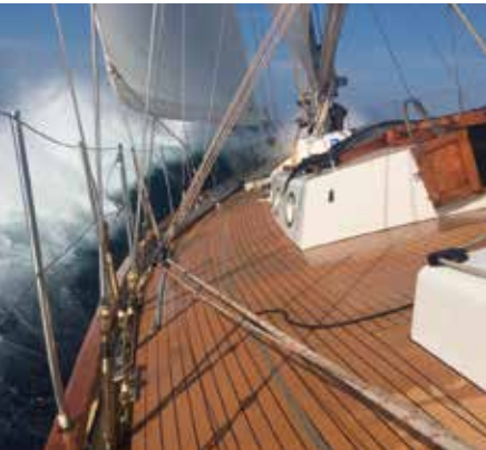
Cork is a surprisingly hard-wearing and high-grip decking material that is also a good insulator. This is a Marinedeck 2000 installation on an Oysterhaven
