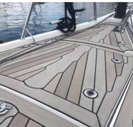
The different colours and textures available in PU extrusions allow for natural-looking decks. Here are two examples from UK-based Permateek, which reflect the two most common trends – a deck that has ‘matured nicely’ by ‘natural’ weathering (left) and a ‘just scrubbed’ teak deck (right)
