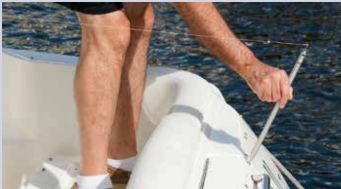
The portable pack includes a pen that allows for accurate measurements within awkward places. The system can also be used for templating windows and canopies
