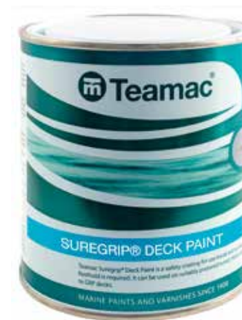
One-pack deck paints have proved a dependable, low-cost and lightweight solution for years. Teamac’s Suregrip and AkzoNobel’s International Interdeck are good examples. Both contain pre-added aggregates that give a roughened surface, and have a coverage of between 6-10m 2 per litre. The basic five-colour choice can be expanded by tinting the white
